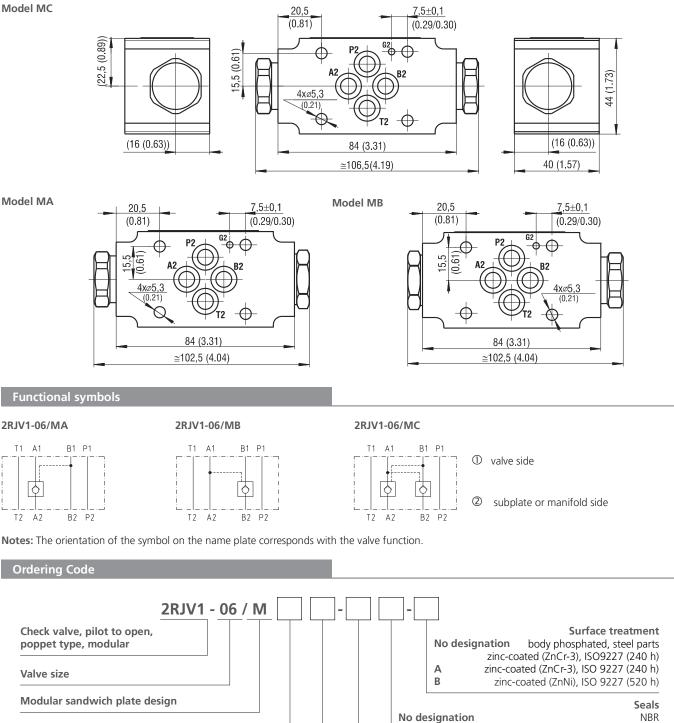
С check valve in line A and B 3: 1 (for all cracking pressures except 2 bar) 3 6 : 1 (only for cracking pressure 2 bar) 6 9: 1 (only for cracking pressure 0 bar and 3 bar) 9 **120** (for pilot ratio 3 : 1)
