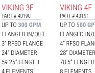
VIKING 4F PART # 40191 **UP TO 500 GPM** FLANGED IN/OUT 4" RFSO FLANGE 28" DIAMETER
