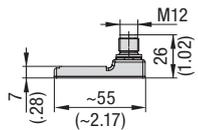
1 Contact opens and 1 contact closes when fluid level drops below contact level
