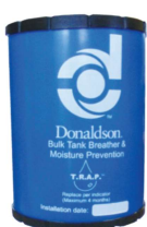
P923075 Urethane 1 1/4" BSP (m) Total Height: 247 Diameter: 176.5 Efficiency: 3µ @ 98%
