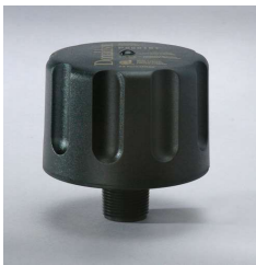
P566151 Glass-filled ABS 1" NPT Total Height: 115.1 Diameter: 114.3 Efficiency: 3µm @ 98%
