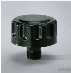
P565857 Epoxy-coated steel 3/4" NPT Total Height: 72.9 Diameter: 80.8 Efficiency: 3µm @ 98%
