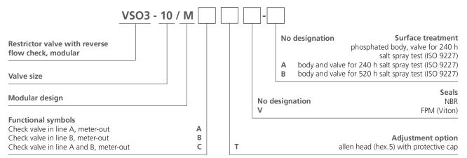
The valves are assembled in meter-out version.
